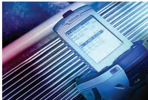
XRF TECHNOLOGY DETERMINES MATERIAL COMPOSITION VERSUS MILL CERTIFICATION TO ASSURE THE RIGHT MATERIAL IS DELIVERED EVERY TIME.
